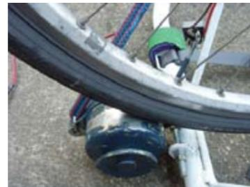
The dynamo is 24 Volt AC, which means we need some extra parts between it and the appliances we want to run (on either 12V DC or 240V AC). The first of these is a Bridge Rectifier (under £5). This converts the AC Voltage into DC. If you had a DC motor/dynamo you'd want a Diode here instead, to prevent current from travelling into the motor and making it spin (~£2). The rectifier is the small grey box in the pictures above (most clear in the central picture).
